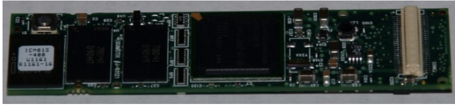
Figure 3.7 - gumstix connex™, view of processor in middle of board
