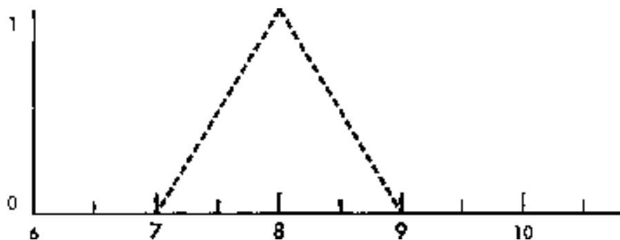
Figure 2.8: An example of fuzzy set of Eightness with a triangular membership function.
