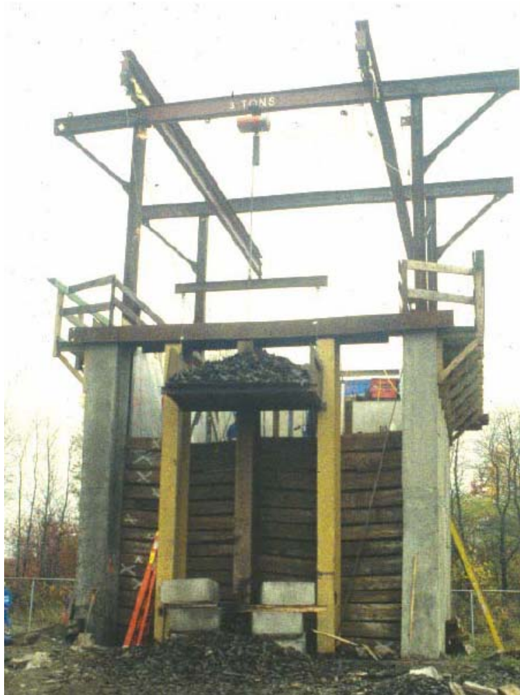
FIGURE 6. Full Scale Retaining Wall Testing for Using TDA as Backfill (4)
