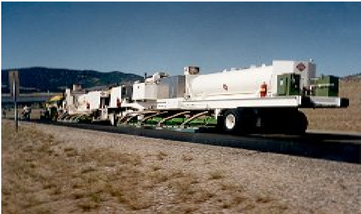
Figure 2 Pyrotech Pyropaver 300E showing the vacuum system for reducing smoke
