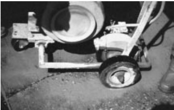
Figure 6.1. Random crack saw.
