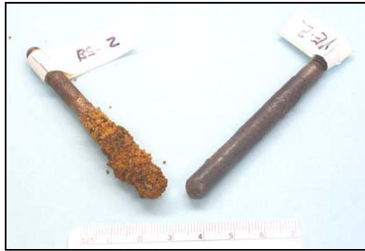
Figure 4. Corrosion on bare steel surface (left) and on enameled steel after 40 days of exposure in salt-water saturated sand. The corrosion of the bare steel cemented sand to the rod.
