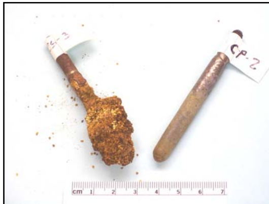
Figure 6. Exhibition of evident corrosion of bare steel surface (left) and not evident on enameled steel containing portland cement after 40 days of exposure in salt-water saturated sand. The corrosion of the bare steel cemented sand to the rod. A powdery, alkaline deposit formed from the hydration of the exposed portland cement.
