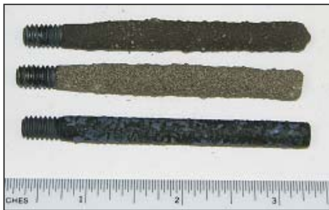
Figure 1. Examples of test rods prepared with various samples of glass frits with an outer coating of portland cement applied to the melted glass.
