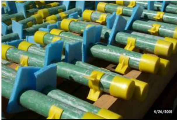
Photo 8. Mn/DOT approved retrofit dowel bar assemblies.
