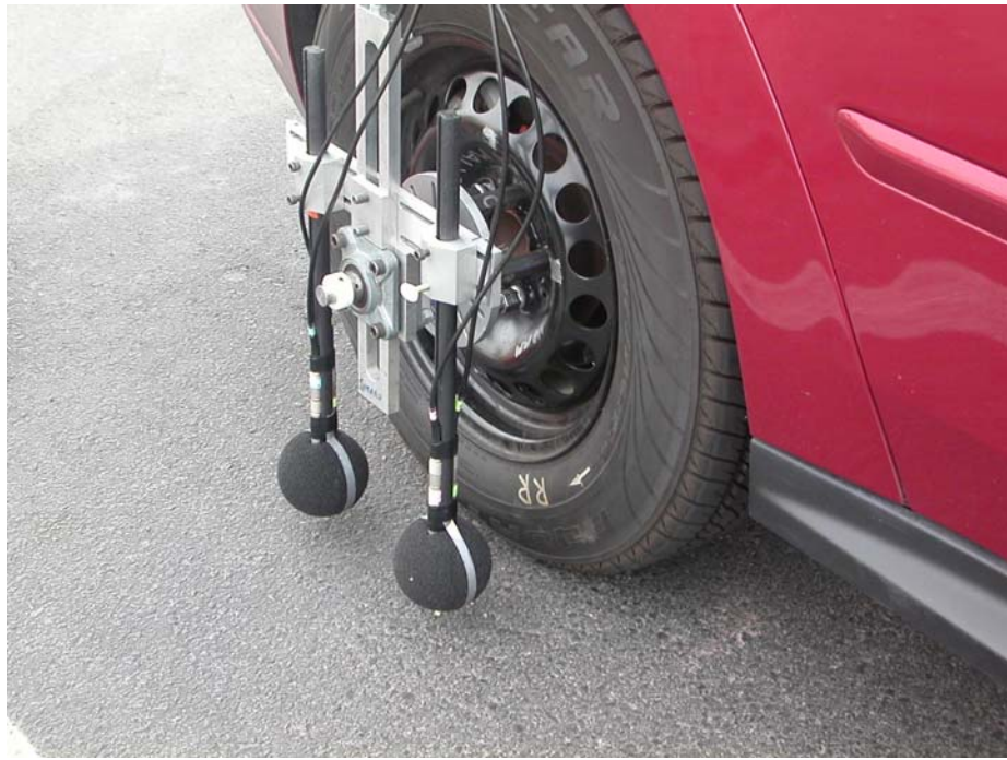
Figure 3. OBSI microphone setup—two-probe system.
