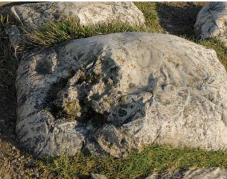
Fig. 5: Cement that was never used as a result of the D-Day invasion. The form is that of the sack in which the cement cured after having been left on the ground after D-Day
