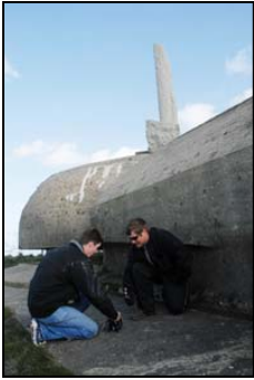
Chad Golden and Andrew Billingsley use Olson Engineering's Concrete Thickness Gauge to determine the thickness of the foundation of the Observation Post at Pointe du Hoc, March 2008.
